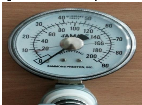
Fig-1 JAMAR hand-held dynamometer
