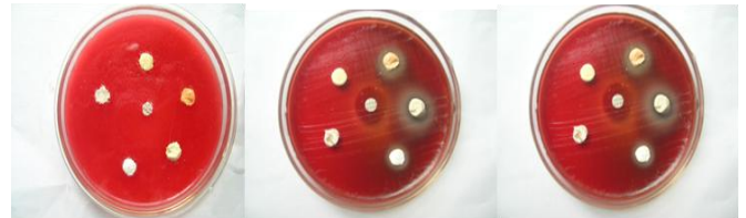
Fig 6 : A sample of sealers impregnated with the zones of inhibition visible at 24 hours and 72 hours
