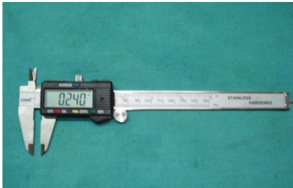
Fig 1. Equipment Used For Taking Measurements Of Anterior Cerebral Artery. (Electronic digital calliper with 300mm operating instructions (0.001mm accuracy))
