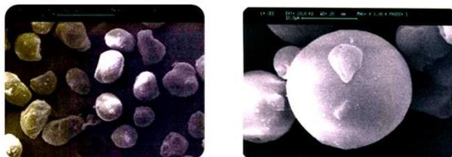
Scanning electron Microscopy shows the particle morphology and density geometrical shape with antigen loaded and unloaded micro particles.
