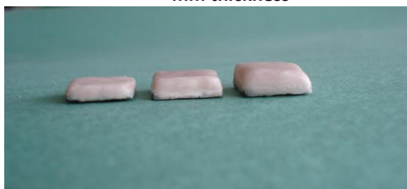
Fig 2: Porcelain fired samples of 1mm, 2mm and 3 mm thickness
