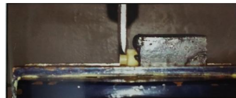
Figure 7: sample sheared with a knife edge on a universal testing machine
