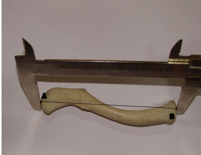
Figure:1. Measurement of maximum length of clavicle(distance between points 'A' and 'B') with vernier calliper
